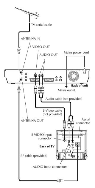
■ To connect to TV's S-VIDEO input and AUDIO input connectors
